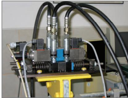
Photo 1. Proportional distributor placed in special holder and bilaterally supported with springs, during testing
