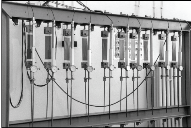
Fig. 3. Test stand for coating material creep
