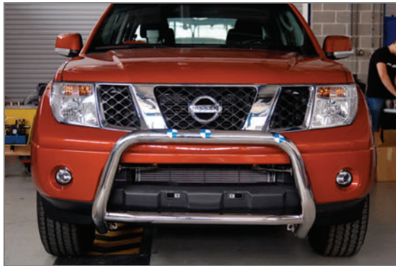
Fig. 8. The Frontal Protection System – 400 mm tubing fitted to the Nissan Navara, front view
