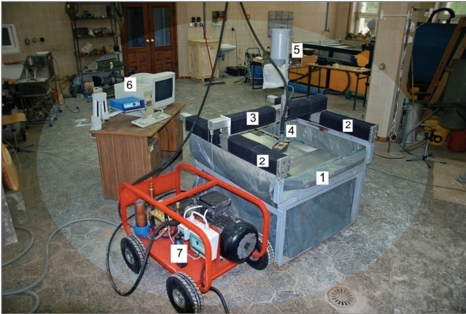
Fig. 2. General view of test stand for spatial material machining with high pressure abrasive-water jet: 1 – frame, 2 – y direction slideways, 3 – x direction slideway, 4 – abrasive-water jet working head, 5 – abrasive feed container, 6 – steering PC computer, 7 – high-pressure water pump type As500/15A
