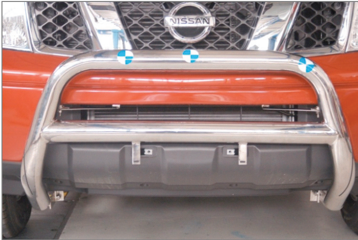
Fig. 15. The frontal protection system – 565 mm tubing fitted to the Nissan Navara, a close-up was made on the points of measurement
