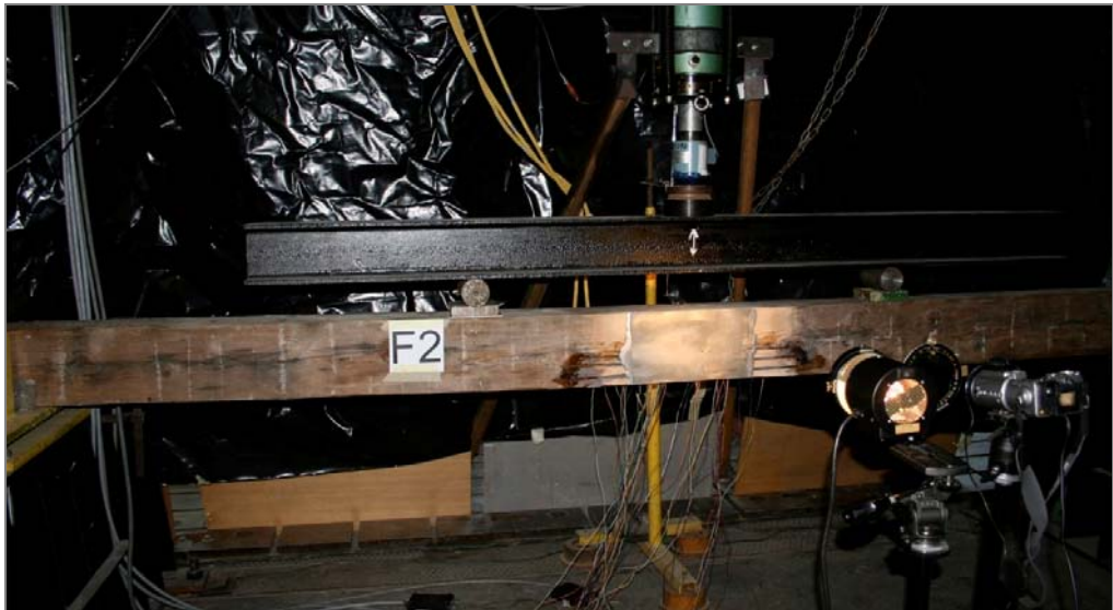
Fig. 3. Beam F2 on testing stand
