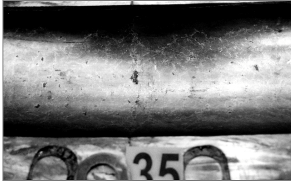
Fig. 4. The surface of the lower race (visible fracturing and minor material losses, minor rolling)
