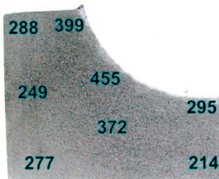
Fig. 6. Race hardness determined by the Brinell method
