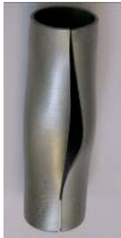
Fig. 10. Panel deformation ( L = 100 mm, \theta = 355^\circ )
