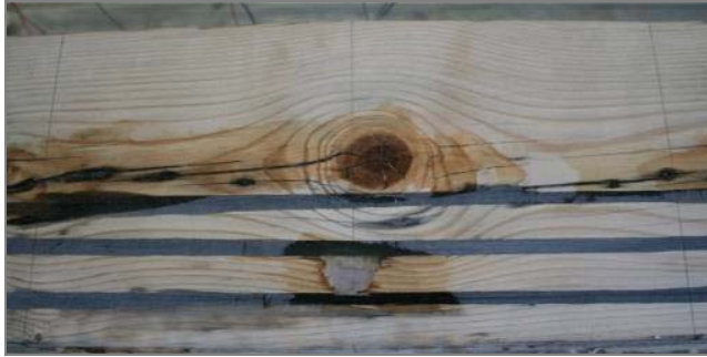
Fig. 6. Surface of beam F2 before photoelastic coating was stuck on [21]
