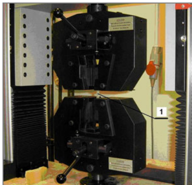
Fig. 5. View of the test bar during tensile process, 1 – test bar
