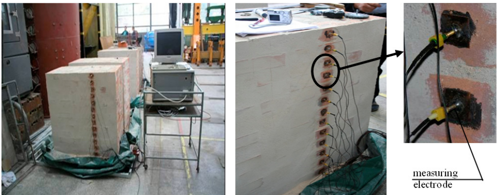
Fig. 10. Test rig with measuring set for electrical impedance tomography
