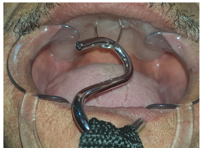
Fig. 3. Digital force gauge used to measure the retention force of the denture base in kilograms-force
