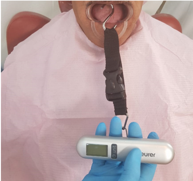
Fig. 4. Pulling force applied downward until the denture was displaced
