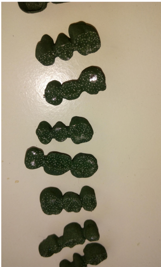
Fig. 1. Co-Cr bridges produced using the direct metal laser sintering (DMLS) method
