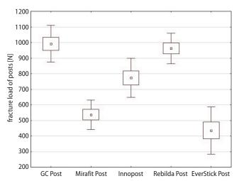
Fig. 4. The flexural strength of posts
