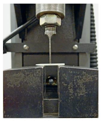
Fig. 1. The post during three-point bending test
