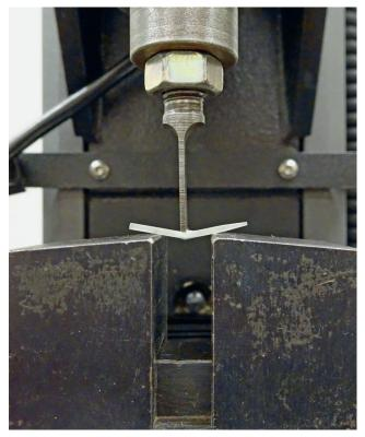
Fig. 2. The broken post after three-point bedning test
