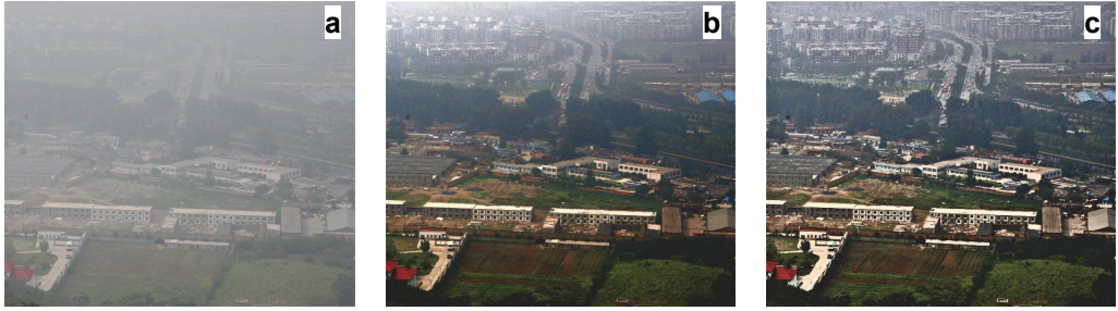
Fig. 3. Original image (a), the result only uses the histogram matching algorithm (b), and final result (c).
