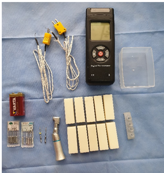
Fig. 3. Laboratory materials (from left to right): a battery, Peeso reamers, a contra-angle handpiece, cords, a thermometer, bone blocks, water, and a surgical guide
