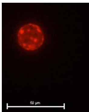
Fig.1. Photo of GUVs made with a microscope Nikon Eclipse TE2000-E with 40× magnification. DiIC 18 was used as a dye. Scale bar 50 μm
