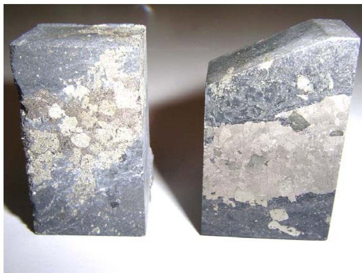
Fig. 3. Prepared black shale working electrodes with mineral rich area.
