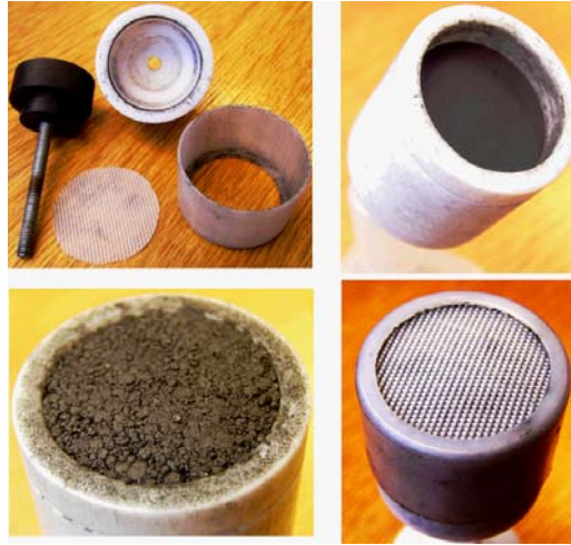
Fig. 4. Construction of the graphite paste electrode
