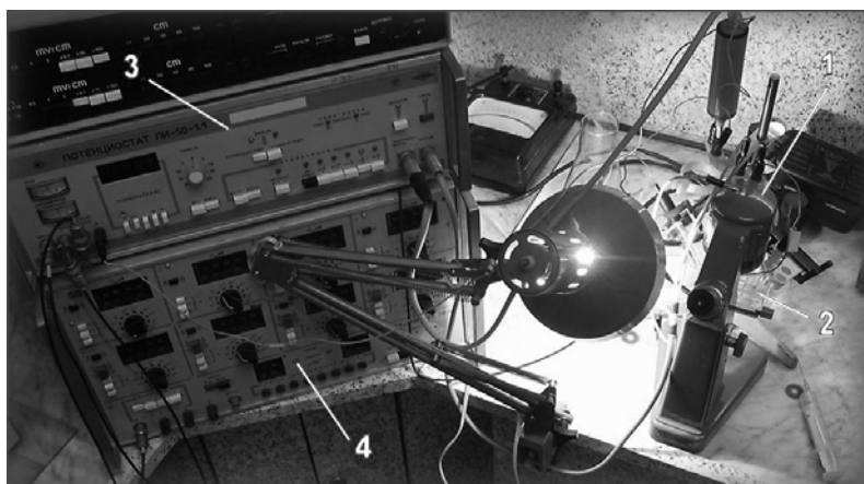
Fig. 1. IT measurements in conditions of electrochemical polarization: 1- the Glembotskii device for IT measurements; 2 - three electrode electrochemical cell; 3 - potentiostat PI-50-1.1.; 4 - programmer PR-8
