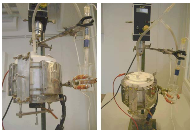
Fig. 2. Modified Avesta cell used in solid sample leaching experiments
