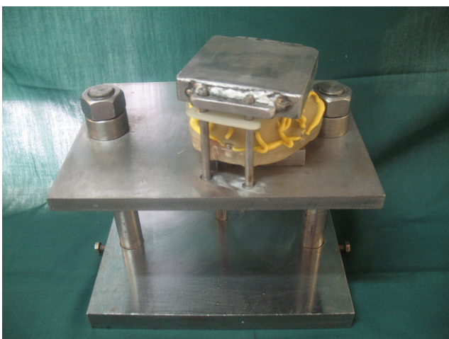
Fig. 6. Metal plate covering the wing during impression making
