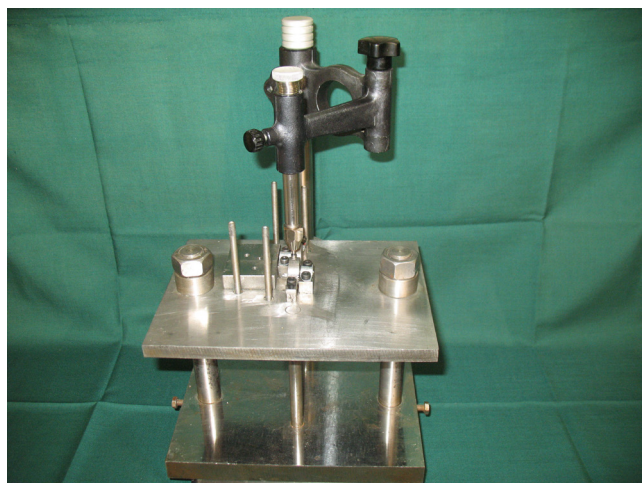
Fig. 3. Accommodating the implant axis to the center of the implant hole by means of a surveyor
