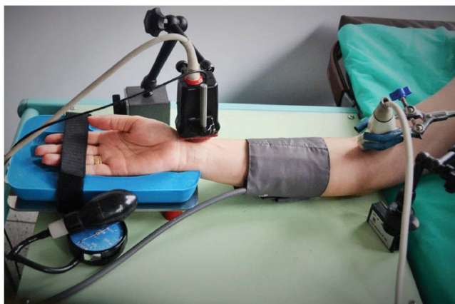
Fig. 1. Experimental setup for simultaneous examining of the flow-mediated dilation in radial and brachial arteries (FMD-RA and FMD-BA) using 20 MHz and 7 MHz linear arrays, respectively
