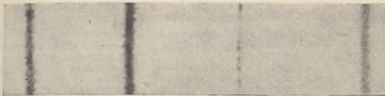
Fig. 2. PORTION OF ELECTRON DIFFRACTION PATTERN FROM CADMIUM OXIDE PARTICLES, SHOWING DIFFERENT LINE BREADTHS FOR 222, 400, 420 AND 422 REFLEXIONS. ENLARGEMENT 16 DIAMETERS
