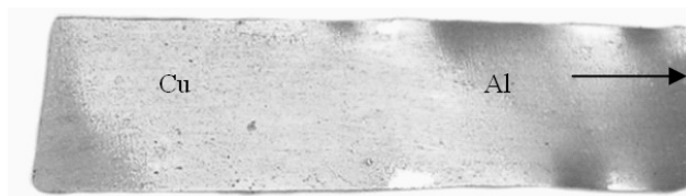
Fig. 6. Al-Cu sample after longitudinal rolling with a small cold work in each pass [4]
