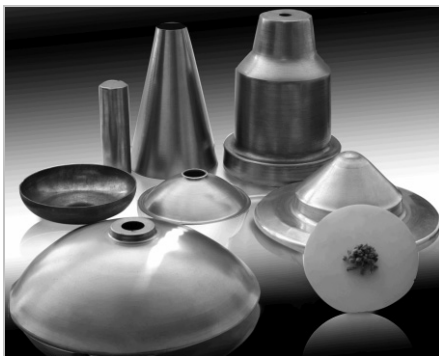
Fig. 1. Examples of spun and flow formed products
