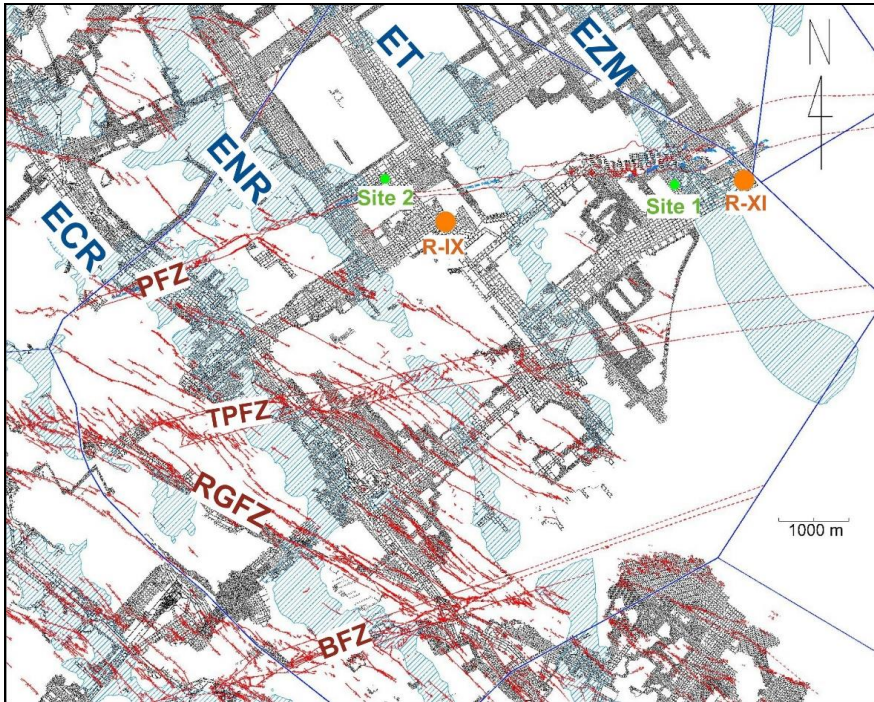
Fig. 1. Overview map of the Rudna mining area against the background of the elevation zones of the top of the Weissliegend (dashed blue), identified tectonic structures and the (red lines) outline of the mine workings (black lines); explanations of abbreviations: ECR – Central Elevation of Rudna, ENR – Northern Elevation of Rudna, ET – Tarnówek Elevation, EZM – Żelazny Most Elevation; RGFZ – Rudna Główna Fault Zone, BFZ – Biedrzychova Fault Zone, TPFZ – Trzebcz-Polkowice Fault Zone, PFZ – Paulinów Fault Zone; R-IX, R-XI – location of shafts)
