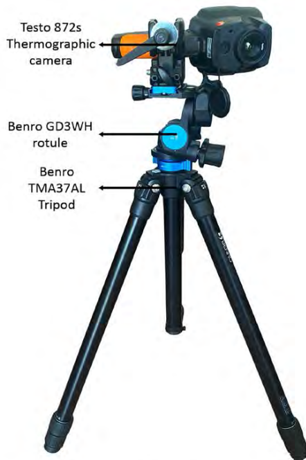
Figure 1: Thermographic camera, rotule and tripod
