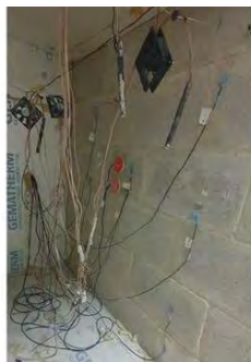
Figure 3: the hot side of the hot box with the sensors installed.
