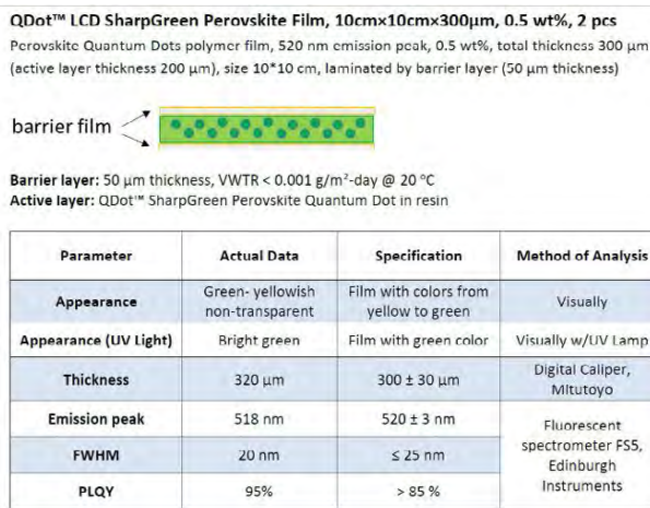
Figure 1. Composition of green perovskite quantum dots polymer films.
