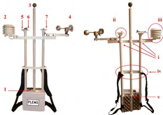
Figure 1: PLEMS sensors and construction details.
