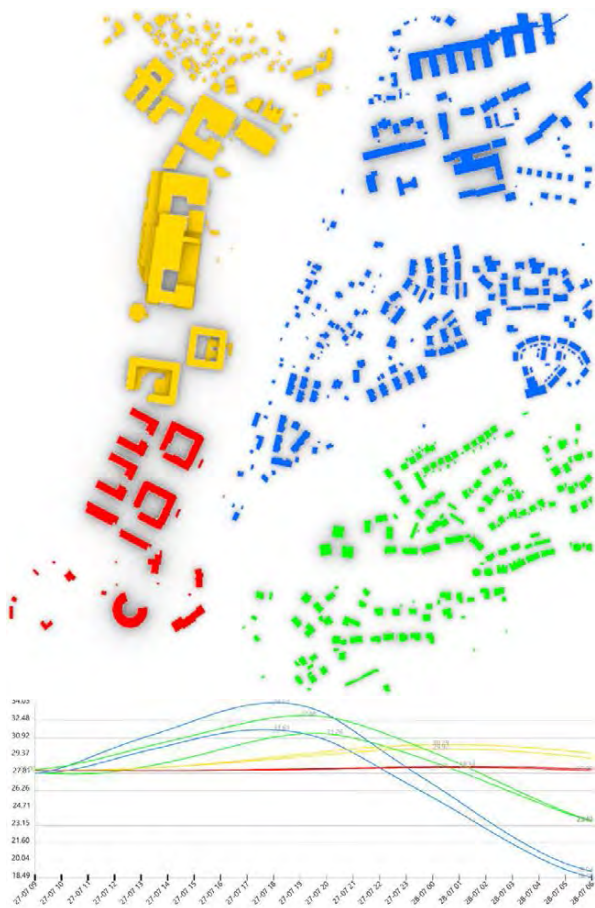
Figure 8: Daily temperature profiles across various building types showing the Influence of construction era and insulation. In red are new residential units, in yellow are new offices, in blue are older family houses built in the 60s, and in green are newer family houses built in the 80s and the 90s in the proximity of forests.
