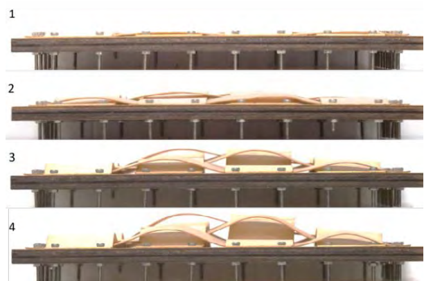
Figure 3: A) Bio-HNV small-scale prototype - Cyclic behaviour between RH = 20%, 50%, 70%. B) Hysteresis Curve of wood veneer swelling during one cyclic test at a constant temperature of 25 C and different RH levels: 20%, 50%, 70% and 90%. C) Humidity responsiveness of the Bio-HNV under different RH levels: (1) 20%, (2) 50%, (3) 70%, (4) 90%.
