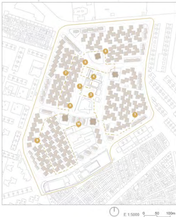
Figure 3: Microclimatic monitoring points distribution in the case study analysis from the field campaign.
