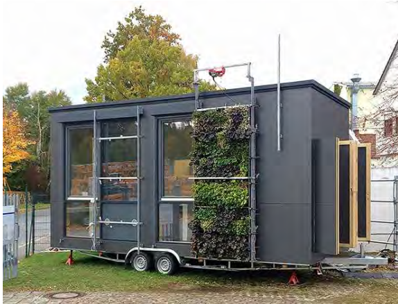
Figure 2: Façade test stand. Reference office with decentralised façade ventilation (DFV) (left) and structure with façade greening "Variant 1" and DFV (right, 10/2019)
