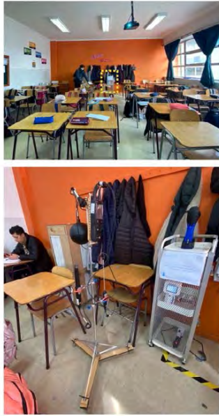
Figure 2: Top image shows the location of IEQ cart at the back of the classroom. Image below, show thermal comfort and air quality dataloggers used for the study
