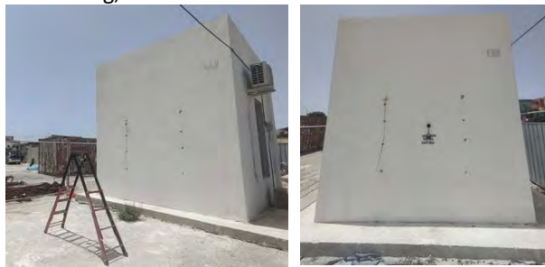
a) Figure 5: The ISO 10140-2:2021 Element Method. a) SLM measuring the outdoor noise. b) SLM on the wall.
