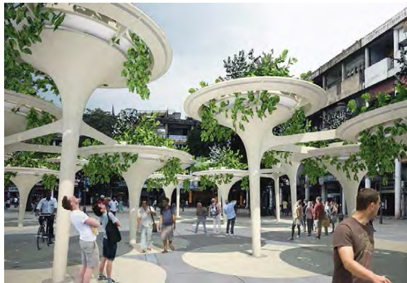
Figure 12: The Xylem, a living roof system developed at CRTKL/Arcadis for outdoor cooling.
