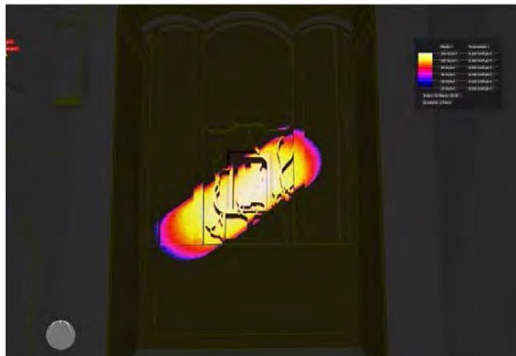
Figure 10: Path of sunlight illuminating the sculptural group representing “El abrazo de San Joaquín y Santa Ana” between 2 p.m. and 3 p.m. on March 20th and September 22nd. Image obtained from a simulation run using Archiwizard V8 software.
