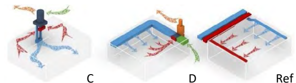
Figure 3: Axonometry of the passive (C), hybrid (D) and active (Ref) ventilation systems in a classroom
