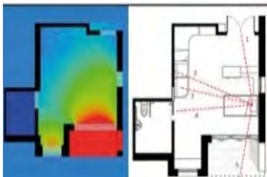
Figure 3: testing room design with daylight contour maps.
