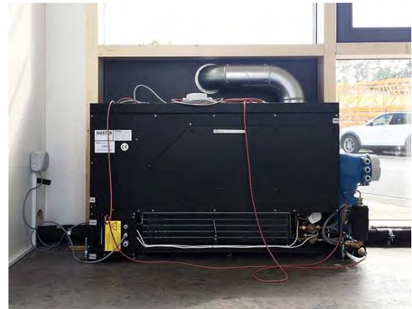
Figure 3: Façade test stand. Reference office with decentralised ventilation unit (DFV)/ room side (09/2019).
