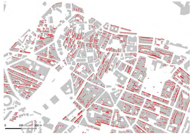
Figure 4 Highlighted exposed perimeters are classified according to their orientation.
