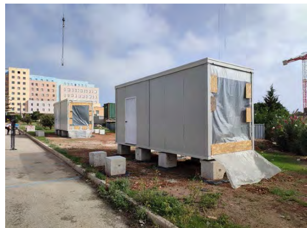
Figure 2: Photos the full-scale, twin test cells installed at the University of Malta grounds.
