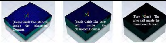
Figure 5: Perspective view of the grids pertaining to the grid sensitivity analysis: coarse grid (318,370 cells), baseline grid (858,680 cells) and fine grid (3,150,219 cells).
