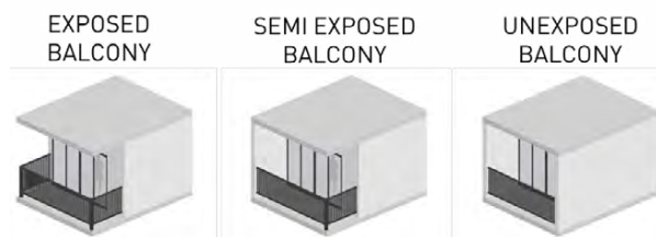
Figure 3: Illustrative scheme showing the different types of balconies identified according to solar exposure.
