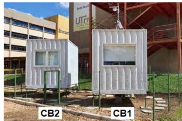
Figure 1: test cell used in experiments (CB1) and reference cell (CB2).
