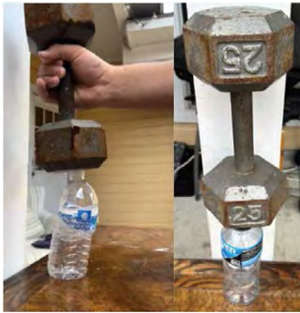
Figure 2: Material selection process of a project – comparing the structural capacity of a water bottle and a sports drink bottle to explain the team’s material finding process (source: Gabe DeLiberty, Leah LeBlanc).
