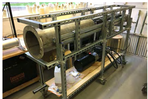
Figure 2: Low-cost, piston-based extrusion machine with hydraulic power unit. Photo: T. Jorgensen, 2020.
