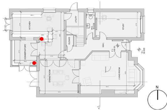
Figure 14: Ground floor plan, Case Study 3, with location of sensors shown in red
