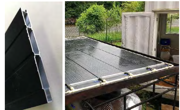
Figure 4: Extruded aluminium profile used in the manufacture of the SR/SC and SR/SC on the supporting platform.
