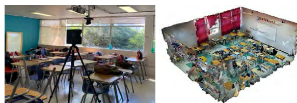
Figure 1: Matterport Pro 2 Rotary Camera & Virtual Scene.
