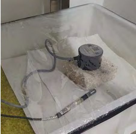
Figure 8: The concrete being tested with disk sensor.
