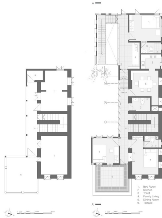
Figure 4: Existing (left) and proposed (right) first-floor plan.
