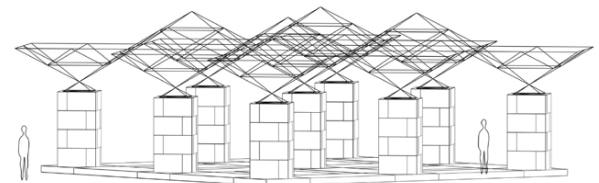
Figure 6: One of the numerous pergola variations can consist of space-frame modular elements.
