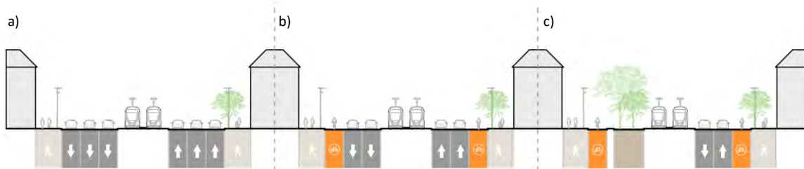
Figure 3: Scenario set-up for Status Quo (a), Bike Lane (b) and Green Promenade Ring (c) Scenarios
