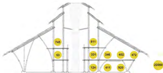
Figure 13: Lux spot measurements (after: section by Ibuku)
