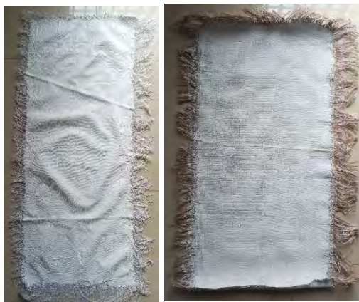
Figure 7: Coated Jute-Polyester fabric on left and coated jute fabric on right.
