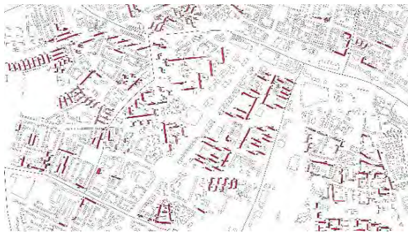
Figure 2: Partial plan of the City of Wrocław. Buildings made of prefabricated panels had been marked with 4 types of shading - author's elaboration..
