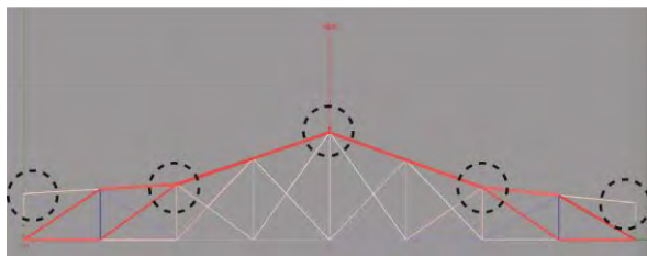
Figure 1: Truss showing the 5 control points of the design generation process. The three in the middle can have their X coordinate adjusted by the designer.
