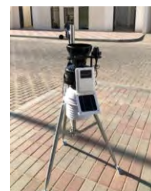
Figure 3. the portable weather station used for the micro-climatic data monitoring
