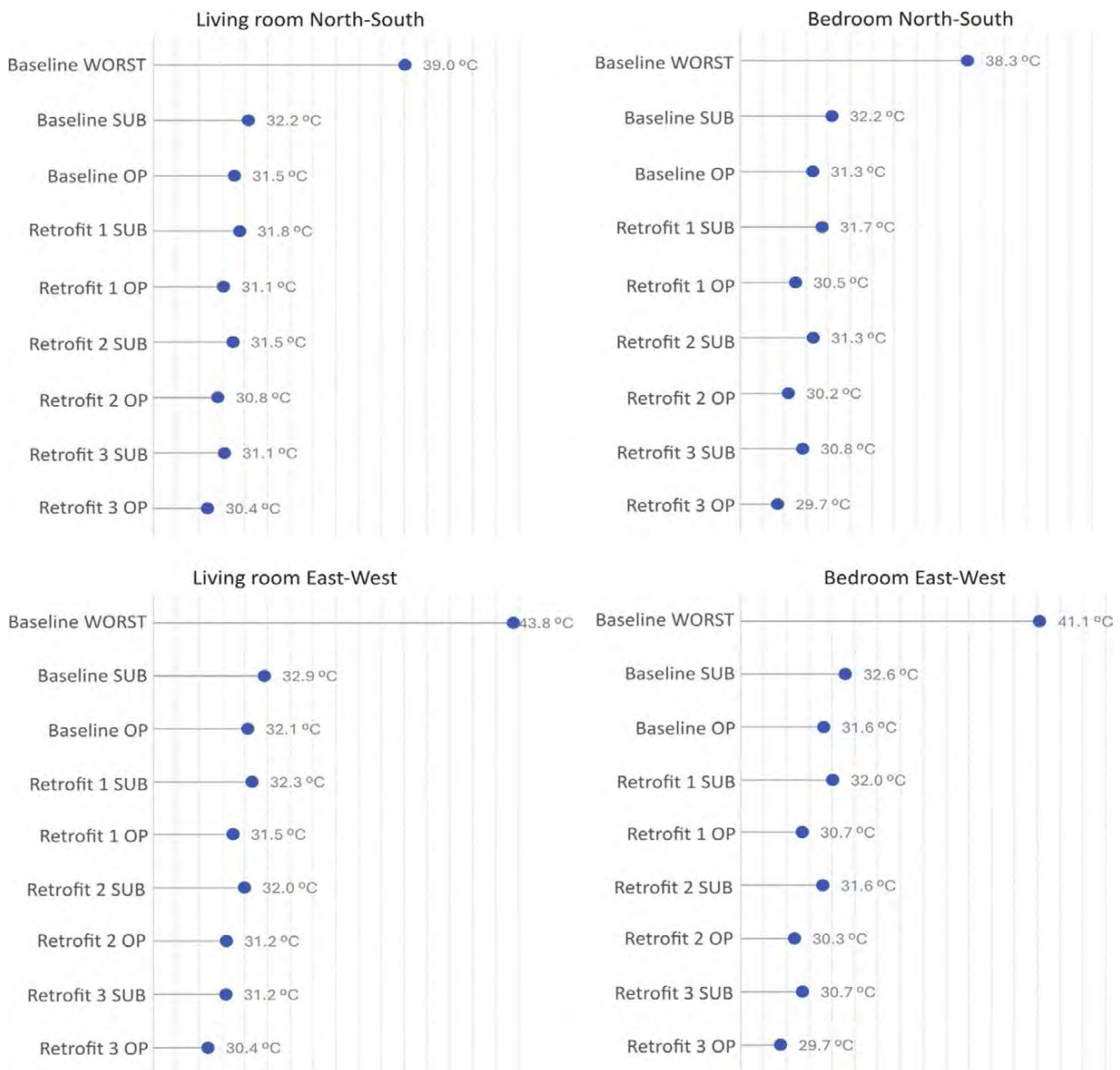
Figure 3: maximum operative temperature during July heat wave
