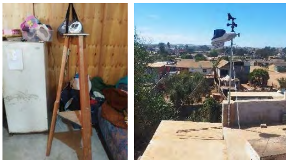
Figure 2: Monitoring equipment on-site: Data logger (left), weather station (Right).
