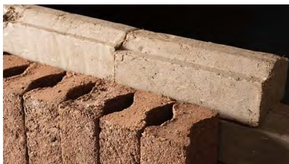
Figure 7: Extruded earth brick design concept, Photo: Simon Regan, 2023.
