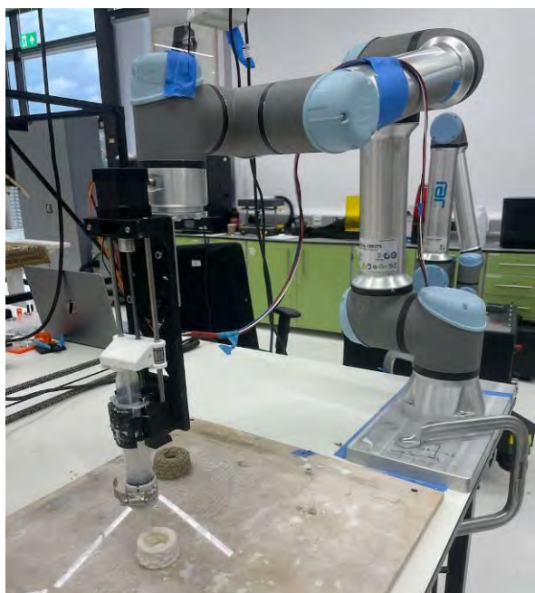
Figure 8: Small scale 3D printing studies of optimal substrates for lichen inoculation.
