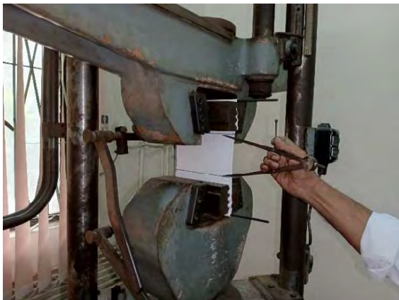
Figure 8: Strip tensile strength testing at Geotech lab, BUET.
