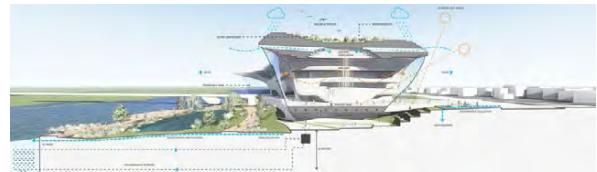
Figure 13: Kaunas concert hall competition proposal by Arcadis that includes an air gap green roof.
