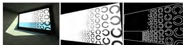
Figure 4: Left: A simulated view generated by CS for view position 0, tint levels of 0, 0, 2 top to bottom. Middle: The resized grayscale format. Right: The detected edges after running the SG-ESSIM algorithm
