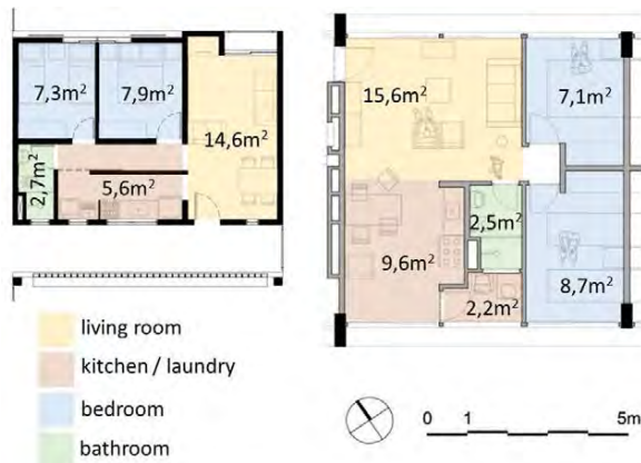
Figures 5 and 6: Example of typical plan of the housing unit of Corruínas (unit type 1) and Jardim Edite (unit type 3).
