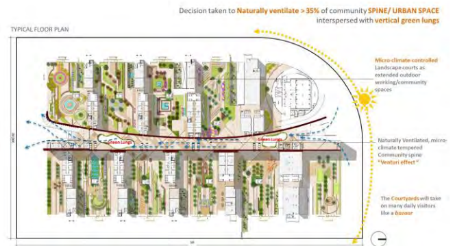
Figure 5: Typical floor plan showing the central spine connecting office towers segregated by landscaped courtyards.
