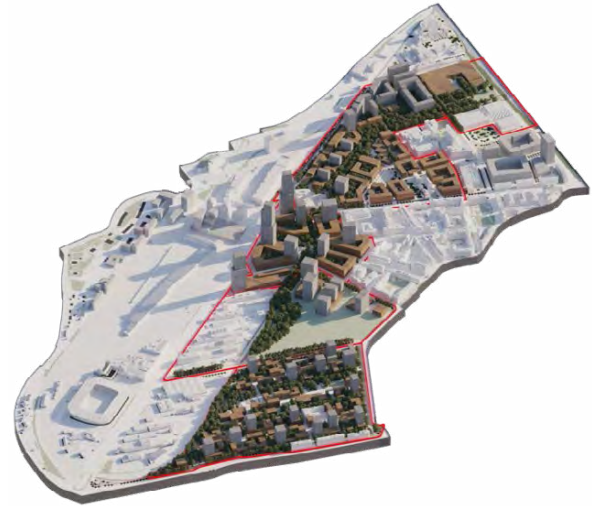
Figure 1: 3D model of public spaces and buildings. White buildings are existing. Grey buildings have dimensions > 30 m and brown ones < 30 m (the latter can be built in wood without major additional investment).
