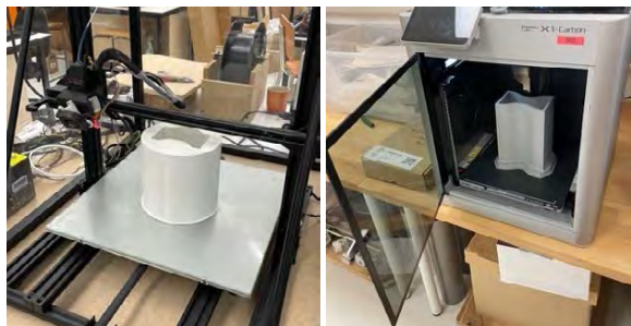
Figure 3: 3D printing of extrusion dies. Photos: T. Jorgensen, 2023.
