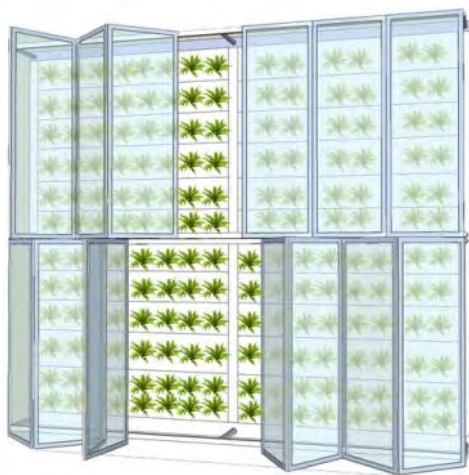
Figure 3: Kinetic shading layer on green façade (Authors)
