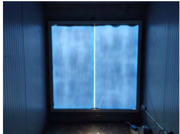
Figure 12: View from the test cell (solar-PDLC OFF; SPD OFF).
