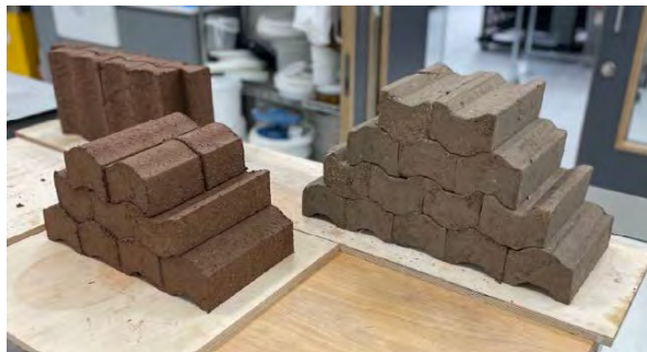
Figure 6: Experiments with interlocking earth brick designs. Photo: T. Jorgensen, 2023.
