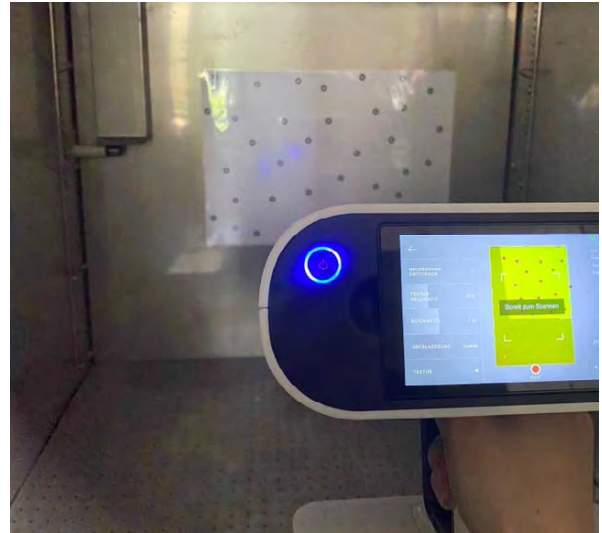
Figure 6: Target points detection of the 3D scanner
