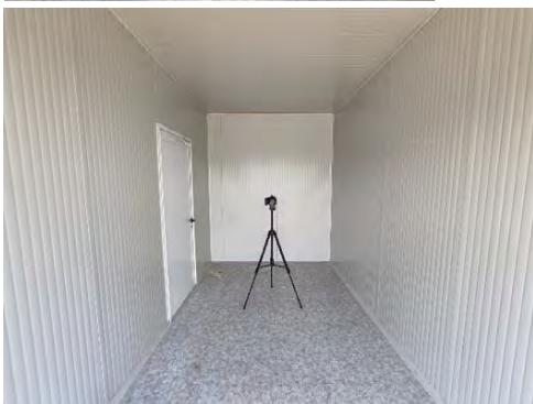
Figure 7: Placement of the luminance photometer within one of the test cells (no glazing installed)
