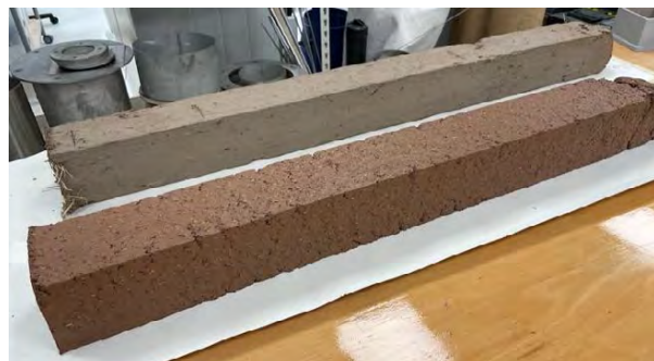
Figure 4: Extrusion tests with both standard cob mixture as well as light earth mixture. Photo: T. Jorgensen, 2020.
