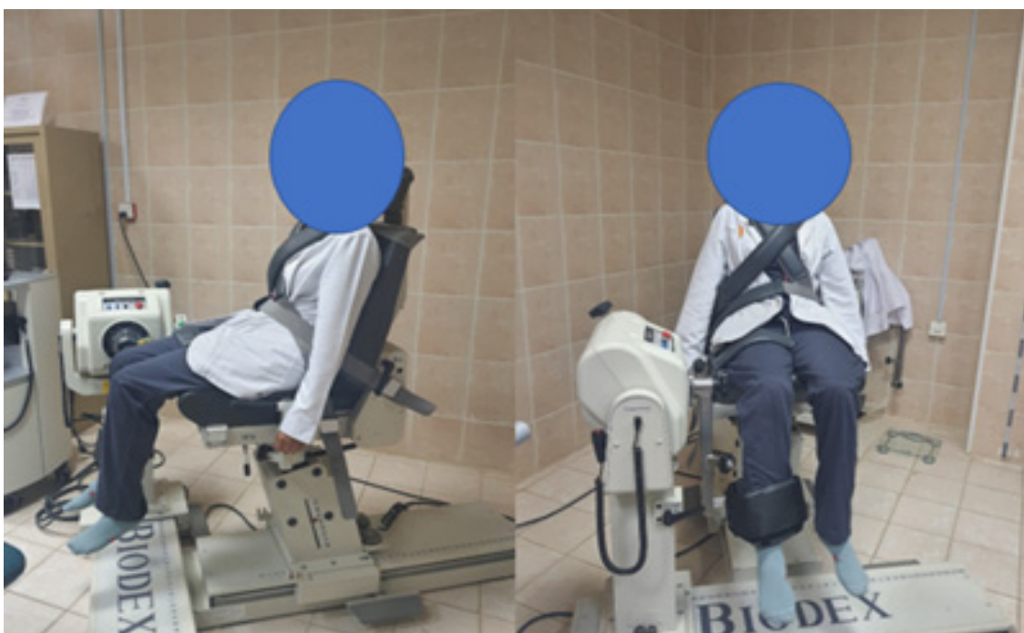
Figure 2. The measurement position for active knee repositioning senses and knee isokinetic parameters
