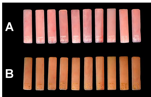
Fig. 2. Conventionally processed polyamide 12 specimens before (A) and after (B) 36 days of storage in coffee
