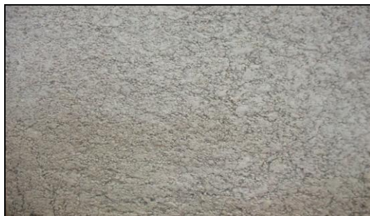
Rys. 2. Widok struktury tynku spienionego Fig. 2. View of the structure of the foamed plaster
