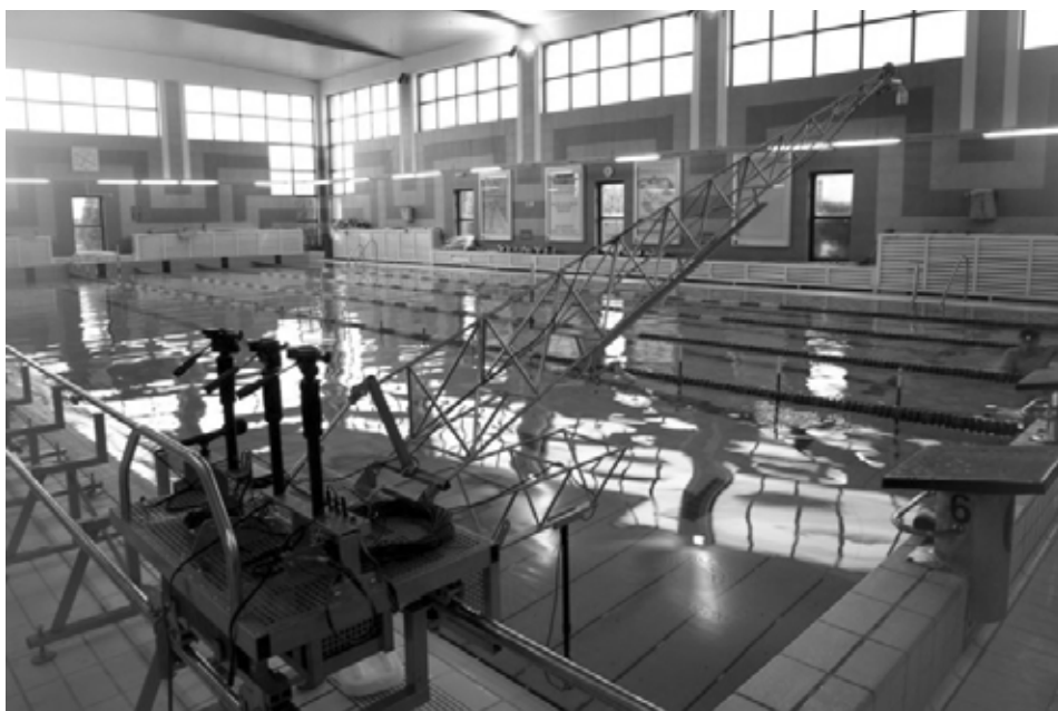
FIGURE 1. Multi-camera swimming technique registration system ( www.l-p-t.pl – website of Laboratory of Swimming Technique)
