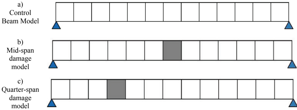
Fig. 2. Beam like structure model used in present study
