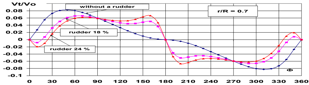
Fig. 7. Tangential component of the nominal velocity field calculated without a rudder and with rudders of different thickness
