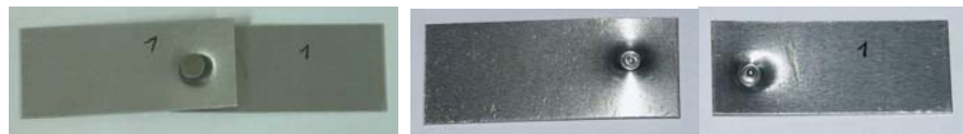
Fig. 4. An example of experimentally obtained SPR joint: left – after forming, right – after shear test
