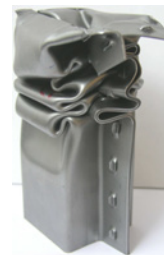
Fig. 10. Failure characteristic of SPJ clinching
