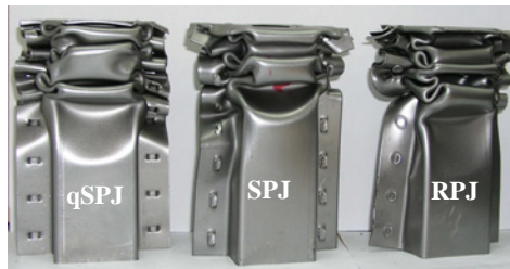
Fig. 9. Collapse thin-walled specimens with pitch of 25 in quasi-static axial crushing
