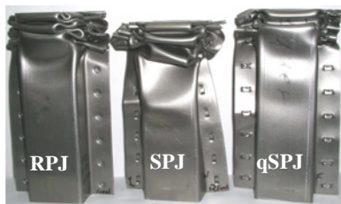
Fig. 15. Collapse thin-walled specimens with pitch of 25 in dynamic axial crushing
