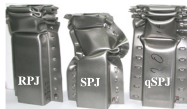
Fig. 16. Collapse thin-walled specimens with pitch of 20 in dynamic axial crushing
