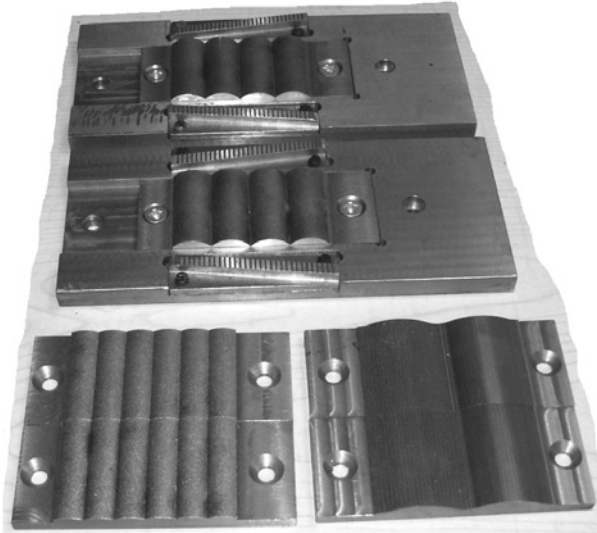
Fig. 7. Tools sets for cross rolling of parts with non-circular cross sections
