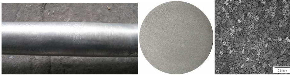
Fig. 12. Billet cast from EN AW-6082 alloy in a horizontal continuous process and the respective macro- and microstructure (from cross-section)
