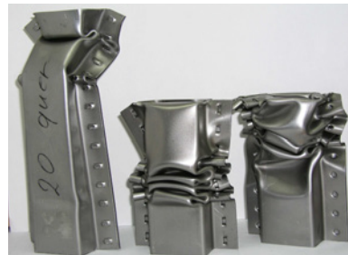
Fig. 12. Collapse thin-walled specimens with pitch of 20 in quasi-static axial crushing
