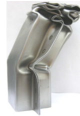
Fig. 2. Global bending of double hat thin-walled sections
