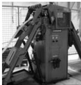
Fig. 2d. Facility with rolls for straightening and running of the strip
