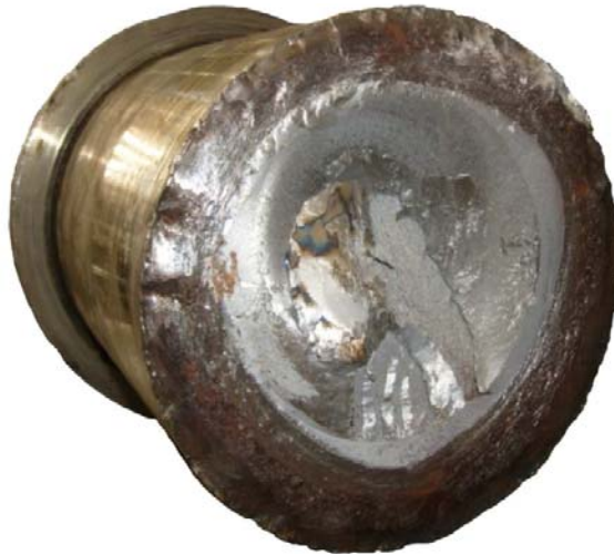
Fig. 1. Damaged shaft – visible wear and plastic deformation
