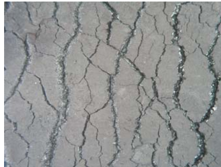
Fig. 8. A grid of cracks on the surface of hot rolled alloy at a temperature of 1200–1100 °C at alloy without spacers
