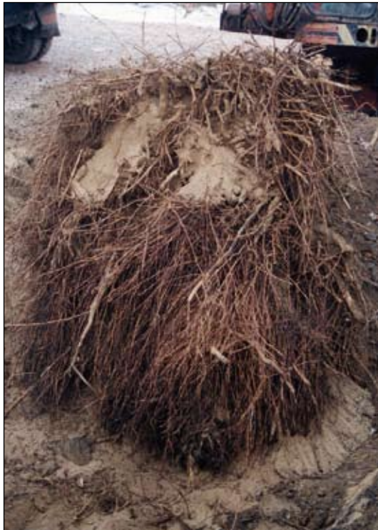
Photo 9. Root systems of trees inside flood banks. Flood bank on Odra – Residential District Zacisze
