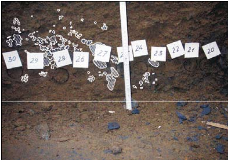
Photo 27. Level 1.25 m below the crown of the bank – marked locations where macro pores were filled with inject
