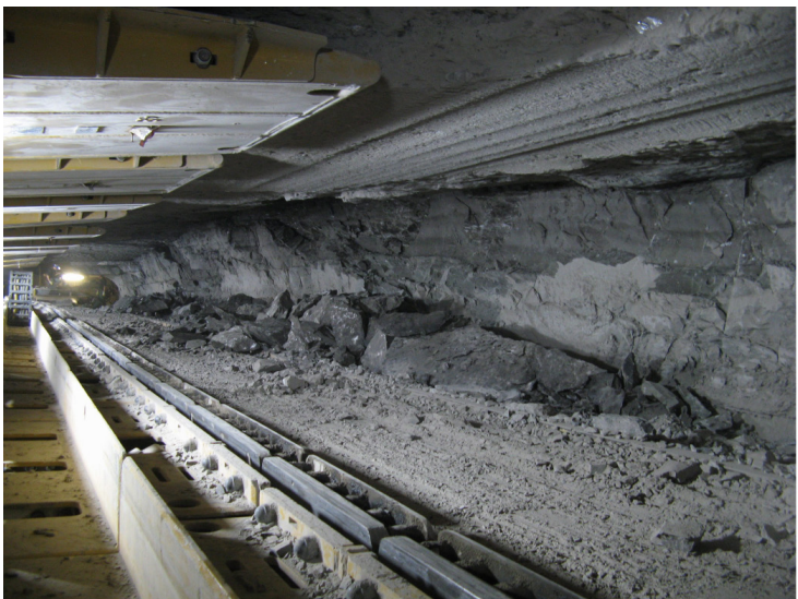
Figure 17: Examples of failures that occurred in the 5A/1 longwall: a, b) roof falls, c) wall spalling.
