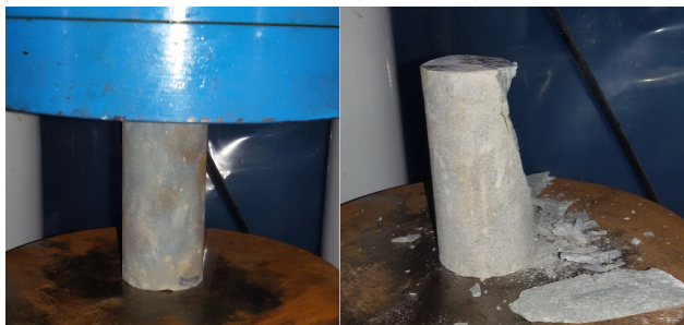
Figure 6: Uniaxial compressive strength testing.
