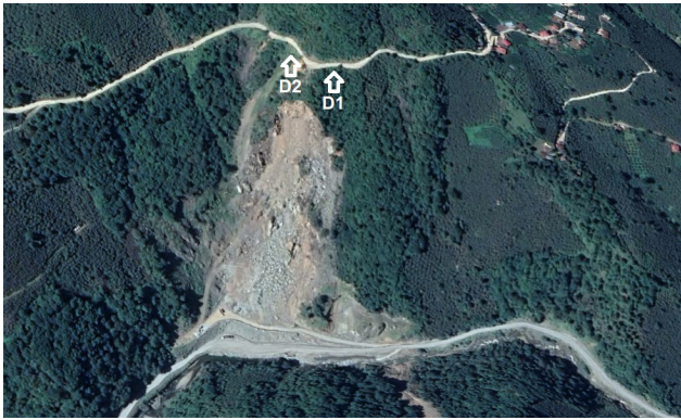
Figure 3: Shown of drilling locations (D1, D2) on the failed Kovanlik quarry.
