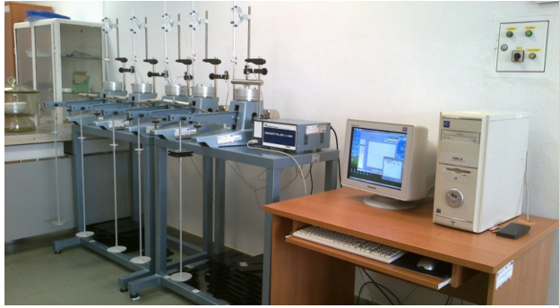
Figure 2: Set of oedometers used for the tests.
