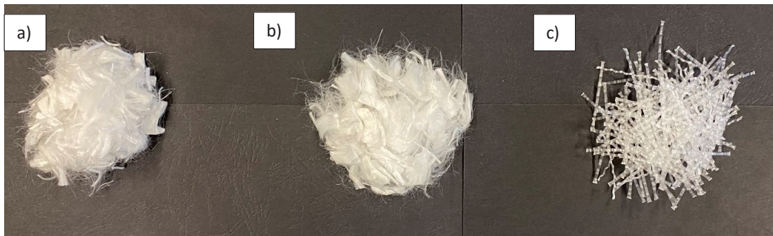
Figure 2: Different lengths (and diameters) of fibres in the amount of 0.2% in reference to the dry mass of the sample that was added to the coarse soil: a) 12 mm (0.030 mm), b) 18 mm (0.034 mm), c) 40 mm (0.090 mm).
