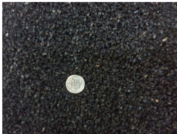
Figure 1: Rubber waste granulate (G) 1–5 mm used in triaxial tests.
