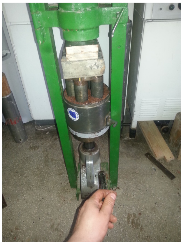
Figure 2: Preparation of specimens from the red clay–granulate mixture.
