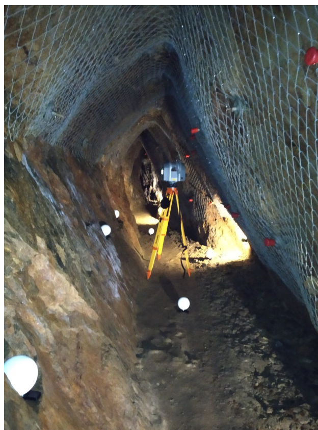
Figure 3: Trimble TX8 laser scanner during measurements in the St. John adit.
