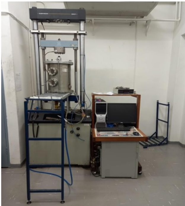
Figure 3: Triaxial testing apparatus.
