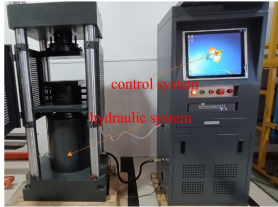
Fig. 3. Microcomputer-controlled servo hydraulic pressure testing machine
