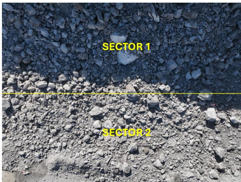
Fig. 6. Division of the muck pile into sectors
