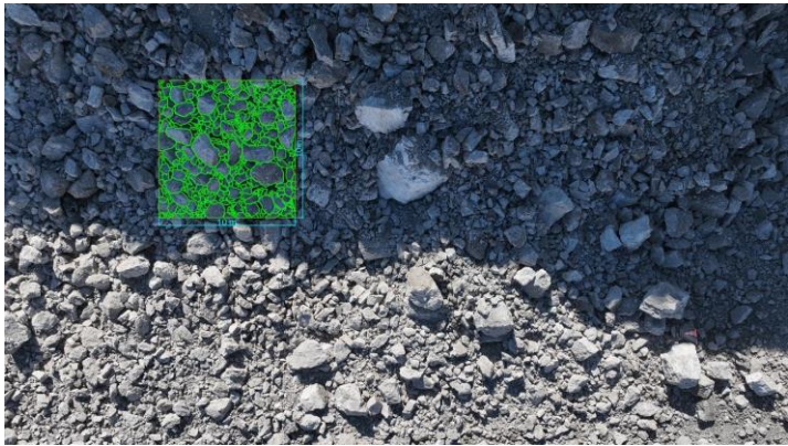
Fig. 2. Selected representative fragment for analysis with dygitize boundaries of grains
