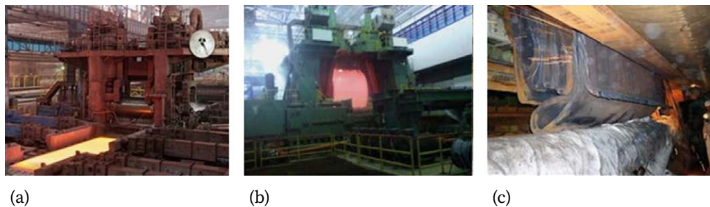
Fig. 7.16. (a) Plate rolling mill; damages caused by front end bending (b) up; (c) down [426]
