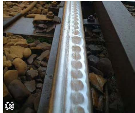
Fig. 2.10. Chatter marks: (a) in unstable boring operation [140]; (b) corrugation of rails [142]
