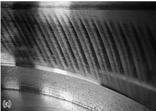
Fig. 2.10. Chatter marks: (a) in unstable boring operation [140]; (b) corrugation of rails [142]
