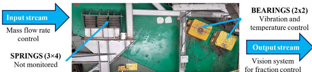
Fig. 4.15. Components of monitoring system on a vibrating screen (non-driven side) with two exciters
