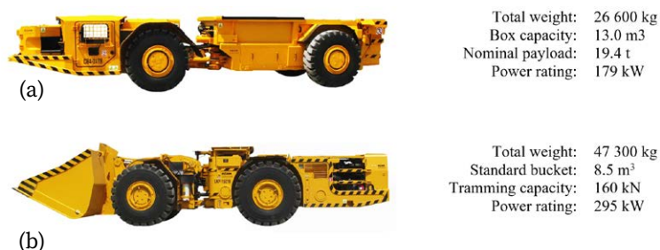
Fig. 2.4. Underground vehicles of KGHM ZANAM (Poland): (a) haul truck (HT) CB4-24TB; (b) load-haul-dump (LHD) machine LKP-1601B
