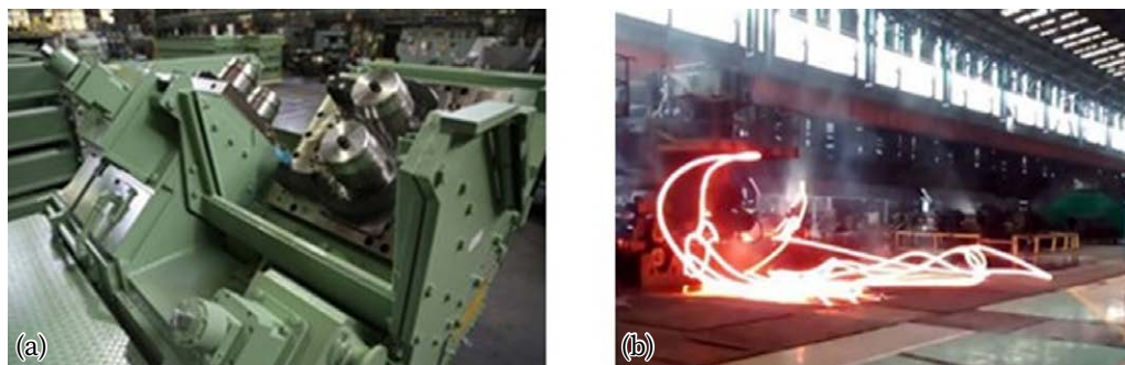
Fig. 2.7. Reducing sizing mill (RSM): (a) gear driveline with a changeable structure; (b) cobbling accident in the mill caused by axial instability of hot rolled rod
