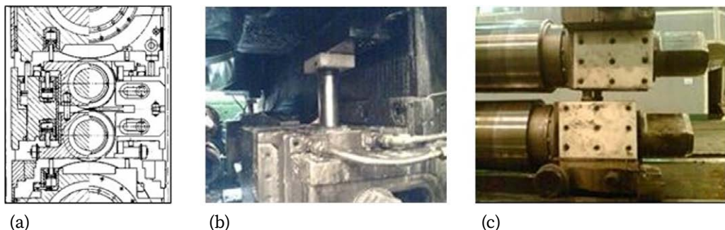
Fig. 7.1. (a) Hydraulic system of the rolling stand; (b) polyamide damping pads on the piston of backup rolls weight balancing cylinder; (c) on the work rolls chocks
