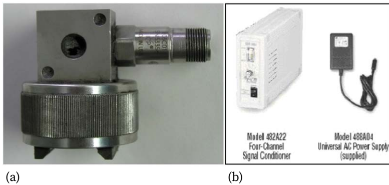
Fig. 8.2. Magnetic mount with adapter for: (a) accelerometer; (b) signal converter
