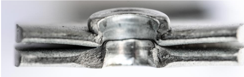
Fig. 2. Clinch joint after fatigue loading
