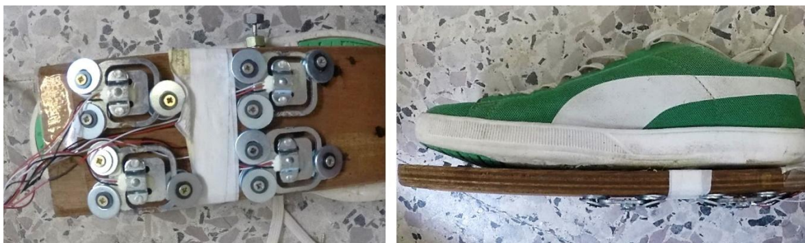
Fig. 1. Views of the right instrumented shoe from below (left figure) and side (right figure)
