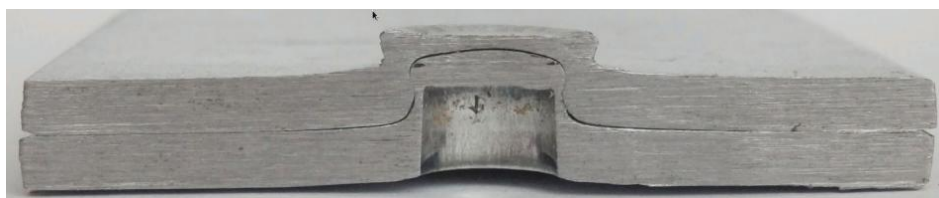
Fig. 1. Clinch joint detail (cut) [1]
