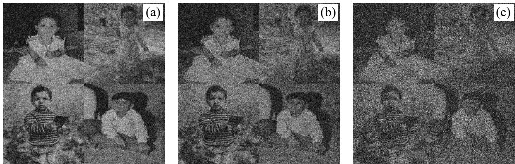
Fig. 8. Noise attack analysis results. (a)–(c) Recovered image with noise strength k = 20 and noise density 0.3, 0.5 and 0.9, respectively.
