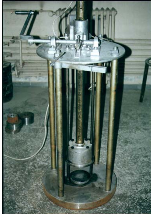
Fig. 1. A photograph of the drop weight apparatus
