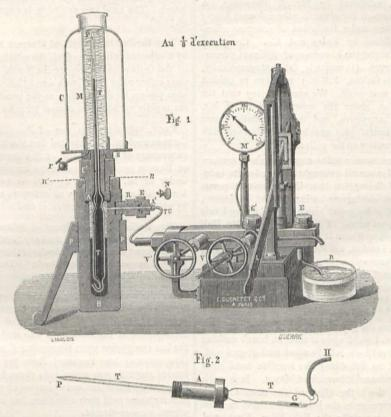
upon leather. The safety-bell-jar C is movable; it is intended to stop the pieces of glass should the tube T be broken. The stop-cock r lets the water flow from the envelope M. The lateral screw with the tube A' is refixed, to which is soldered the small metallic tube TV, by which pressure is introduced.
