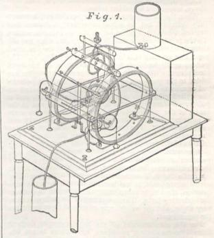
bridge has designed an electro-dynamometer through which large currents may be transmitted and directly measured (*Proc.* Am, Acad. Arts and Sci., October 9, 1878). This instrument works well and gives good results.
