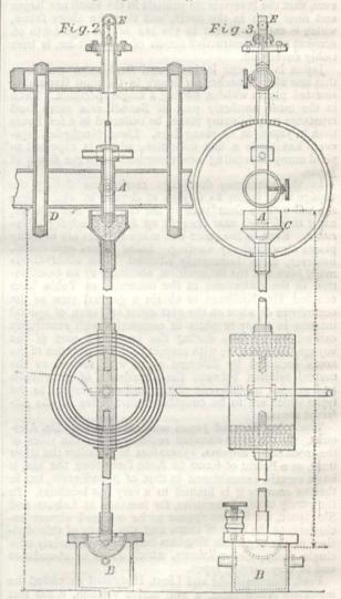
from measurement, and l is a known distance. With the instrument in question, C was found by passing the same currents through it and through Trowbridge's dynamometer, the constant of which was accurately known.
