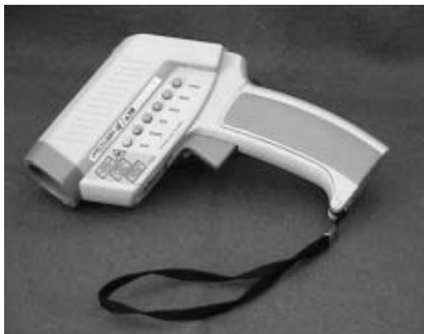
Rys. 4.3. Pirometr Thermopoint TPT 64plus
