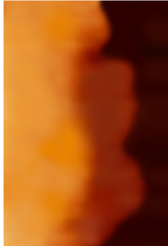
Figure 1.4: Single-layer graphene visualized by AFM. Narrow ( \simeq 100 nm) graphene stripe next to a thicker area. Colors: dark brown corresponds to SiO 2 surface, bright orange \sim 2 nm, light brown \sim 0.5 nm - the high of a single layer. Reprinted from supporting materials to Ref. [28].
