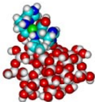
Fig. 5. Molecular model of Cu-L-histidine complex covalently anchored to silica gel via the reaction of amino group of one amino acid and the 3-chloropropyl functionality of the silica gel
