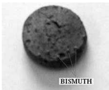
Fig. 9. Decomposed tablet made of mass No. 5 after a hazard in a reducing atmosphere
