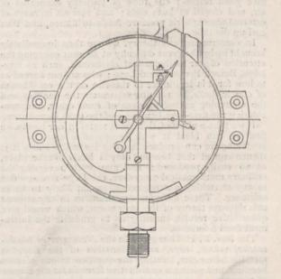
tube is screwed to a pipe which communicates with the liquid whose pressure is to be measured, while the other end is closed and joined by levers and racks to a shaft and a pointer, which traverses a dial on a box in which
