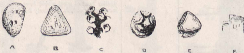
FIG. 3.—Preparations for the microscope of diamonds and other forms of carbon obtained from carburised iron.
