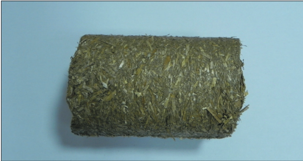
Fot. 4. Brykiet z mozgi trzcino- watej ( P. arundinacea ) Phot. 4. Briquette made of reed canary grass ( P. arundinacea )
