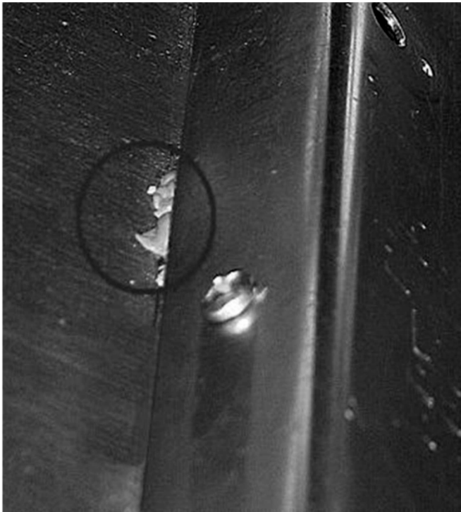
Fig. 1. Situation of the sausage-separator before starting production but after cleaning. Inside the circle product residues are demonstrated
