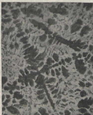
FIG. 6.—Cu 80 per cent, furnace-cooled, \times 33 . V.
