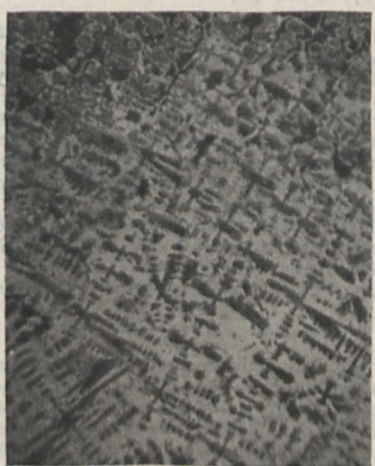
FIG. 8.—Cu 80 per cent. \times 33 . V.
