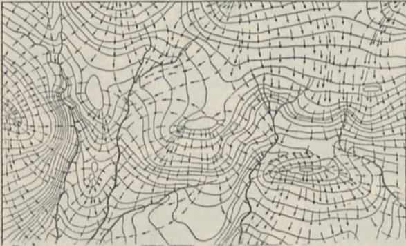
FIG. 1.—Contour Map showing position of water table (continuous lines), supposed lines of motion of ground water (arrowed lines), and the thalwegs or drainage lines (heavy lines).
