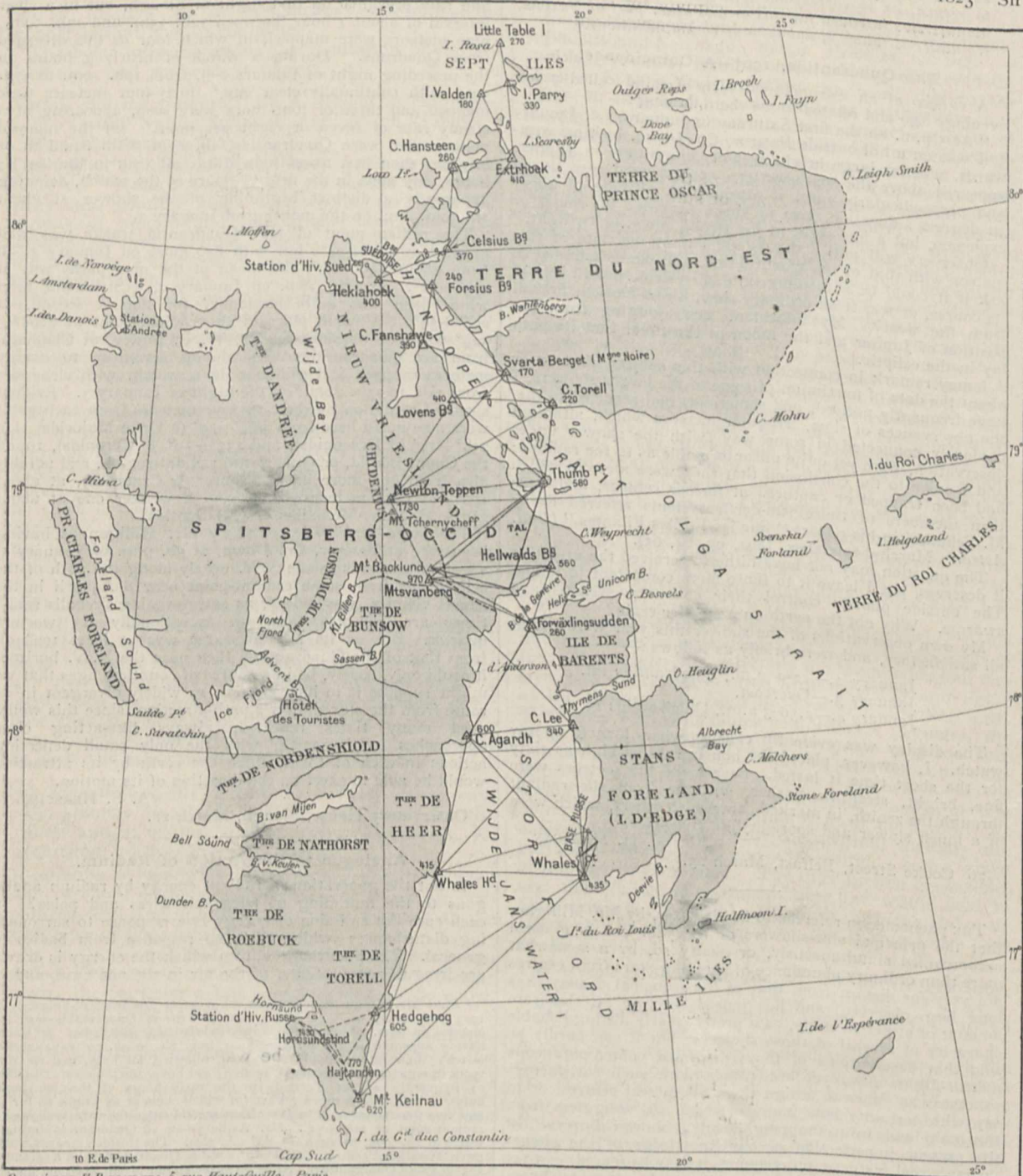
FIG. 1.—Triangulation at Spitsbergen, for the measurement of an Arc of Meridian.
